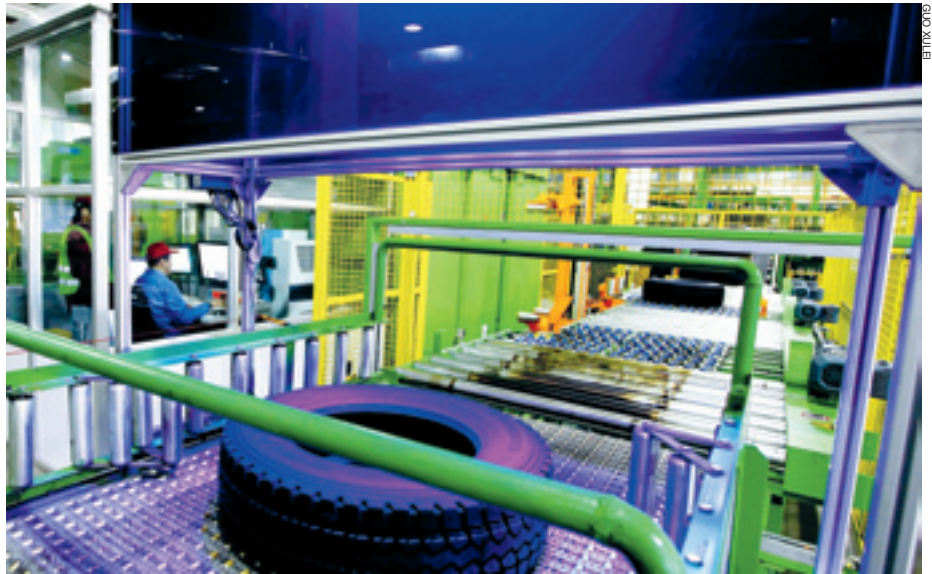
A TIRE HUB A tire receives a quality examination under an x-ray in a workshop of the Shandong-based Triangle Group. East China's Shandong Province has been promoting the competitiveness of tire makers, and its tire exports in 2011 totaled $7.83 billion, accounting for nearly 50 percent of the national total
