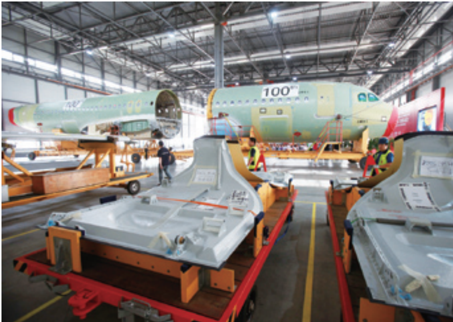
ASSEMBLING AIRBUS Workers check parts for the 100th Airbus A320 aircraft in the final assembly line in north China's Tianjin on June 13. The aircraft will be delivered by the end of the year
